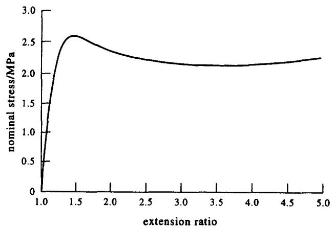
Figure 5 Typical nominal stress-strain curve for a necking polymer, with the maximum corresponding to the onset of necking and the minimum to the natural draw ratio
